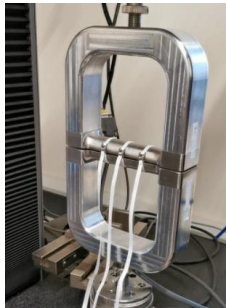
Picture 2. General view of test setup fixed with three Ortholox® UHMWPE Sternal Cerclage Band System
